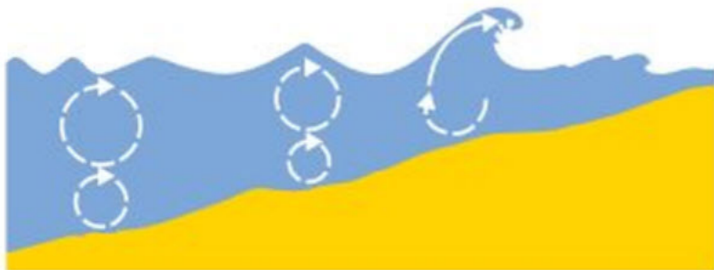
▲ Figure 1 The motion of water in a wave.
