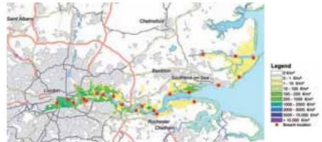
▲ Figure 20 The cost of flood damage in 2050 after a flood similar to the 1953 storm surge if sea levels continue to rise and flood protection is not improved. Red dots show where coastal defences would be breached.
