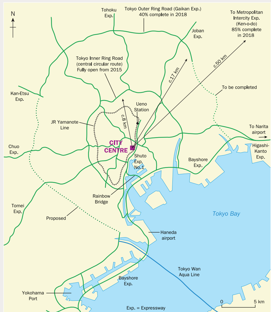
Figure 3 Tokyo: expressways, ring roads and other transport infrastructure, 2019 Source: Adapted from Tokyo subway map, Tokyo Metropolitan Government
